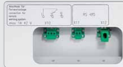
RS485-Interface/Connection for the remote warning system
